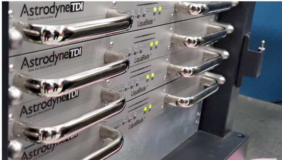
**ADTI's 1U high LiquaBlade™ power module assembly provides three power conversion channels, each rated at output power of 5.5kW for a total module power of 16.5kW.**
